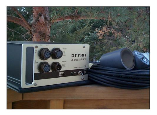
The Deltaflex is a fourth generation acoustic flowmeter and data recorder designed to measure direct velocity, reflected velocity, stage, discharge, temperature, salinity, speed of sound, receiver gain, and the ratio between the reflected and direct velocities.
